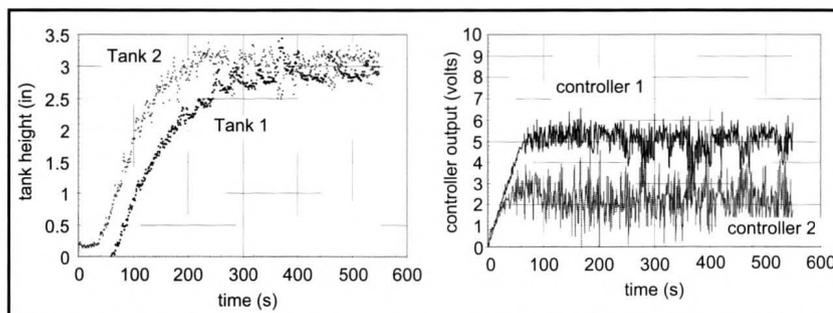
**Figure 10.** Responses to decentralized control with setpoint heights of 3 inches in a strongly interacting system.
