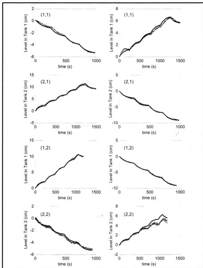
**Figure 3.** Model predictions plotted with experimental data for the four elements of the transfer function matrix: data used to fit model (left), data used to verify model (right). The row and column numbers are reported in the upper-left-hand corner.
