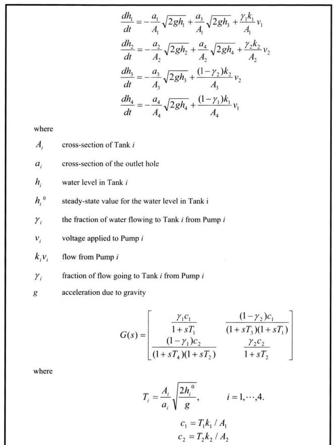
Figure 2. Physical models for quadruple-tank process.<sup>[3]</sup>
