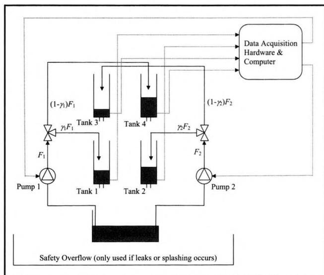
**Figure 1.** Schematic of the quadruple-tank process apparatus. To simplify the figure, not shown are a tube between Tank 3 and Tank 1, a tube between Tank 4 and Tank 2, a tube from Tank 1 to the water reservoir, a tube between Tank 2 and the water reservoir, and a lid on the water reservoir. These tubes and lid are used to reduce evaporation.
