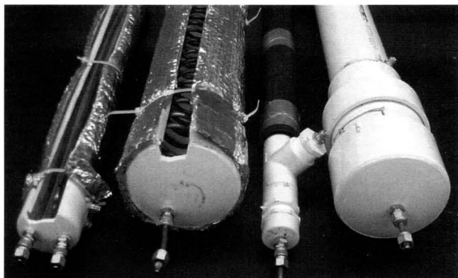
Figure 3. Examples of student-built heat exchangers and construction materials. At the left are examples with the shell cut away to reveal a multipass and coiled-tube design. At the right are double-pipe and shell-and-tube heat exchangers.
