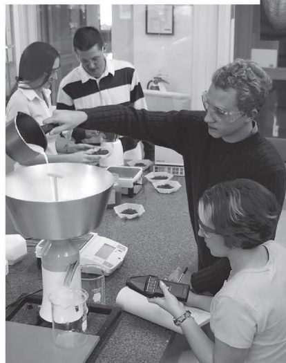
▲ Fluidized bed for polymer coating experiment in the freshman clinic.
