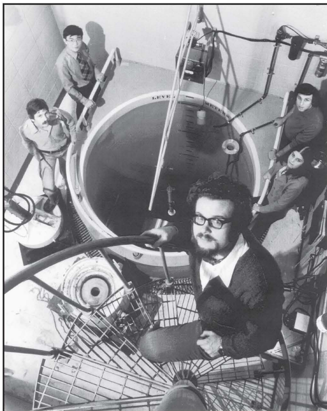
Professor Carl Gryte (on staircase) with Isao Noda (top left) and other doctoral students installing the Cobalt-60 radiation source used in polymer research (about 1971).
