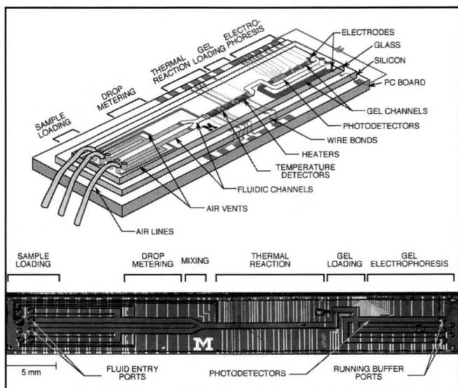
**Figure 1.** An example of a Lab-On-a-Chip device. This is a DNA analysis system devised by Mark Burns and associates.<sup>[1]</sup> Various “unit operations” including metering, mixing, reactions, separations, and detection are combined in a single device.
