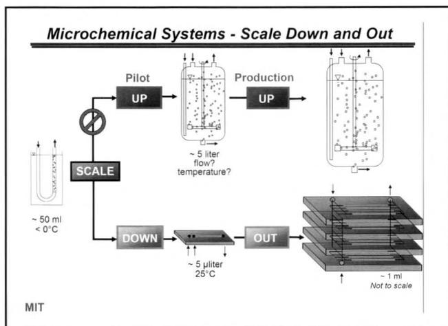
**Figure 2.** Klavs Jensen’s concept for a new paradigm in chemical process development that utilizes the multiplexing capabilities of MEMS technology to carry out integrated synthesis and separation operations in the same unit.
