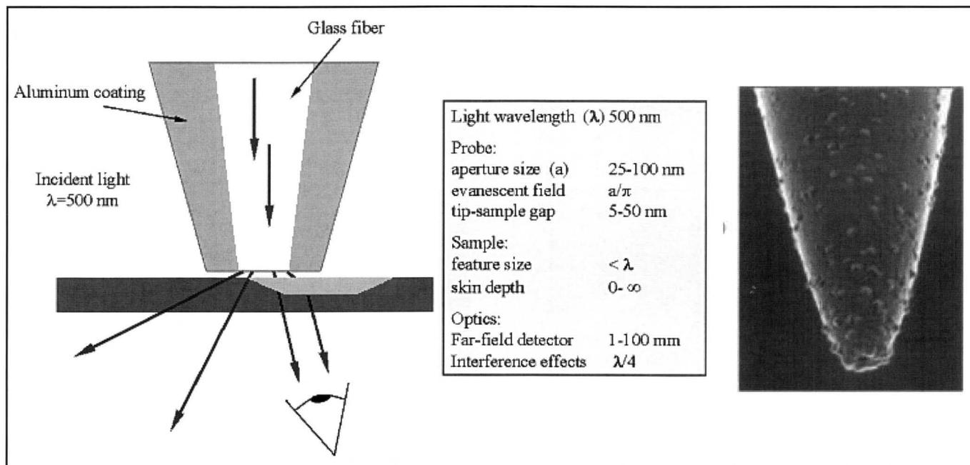
**Figure 4.** Operational characteristics of near field microscopy (left). Close-up of the optical scanning probe (right). This is one of the devices that will allow the visualization of structures within living cells and their behavior.
