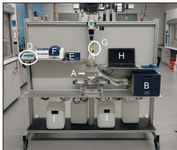
Figure 3. KIN experimental apparatus: One-liter, jacketed glass reactor (A) with temperature-controlled recirculator (B). An overhead agitator (C) mixes the reactor with the agitation speed set by a motor controller (D). A peristaltic pump (E) circulates reactor contents to the in-line spectrophotometer (F). Absorbance and the reactor temperature from the thermocouple (G) are recorded and displayed on the laptop (H). Waste is drained into containers (I).
