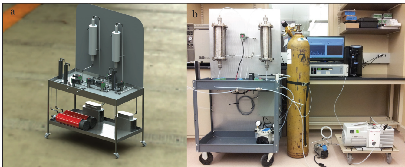
Figure 2. Vacuum swing adsorption system built by undergraduates using systems engineering methods: (a) computer aided drawing of the system to be built; (b) the completed vacuum swing adsorption system.
