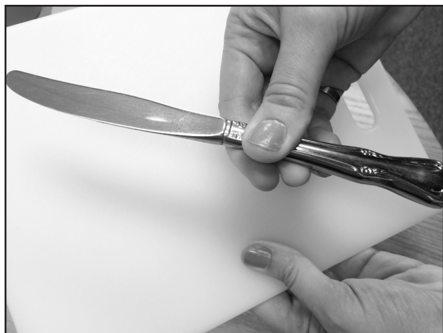
Figure 3. Two items from the Human Thermometer activity: The stainless-steel knife feels significantly “colder” than does the plastic cutting board, although both are at room temperature.
