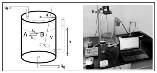
Figure 3. Schematic of the CSTR along with a first-generation prototype in the lab setting.
