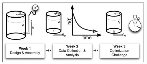
by varying inlet and/or outlet flow rates, liquid accumulation within the tank occurs. Subsequently, as the concept of component balances is added to the existing understanding of mass balances, a "source" term is added to account for chemical reactions.
