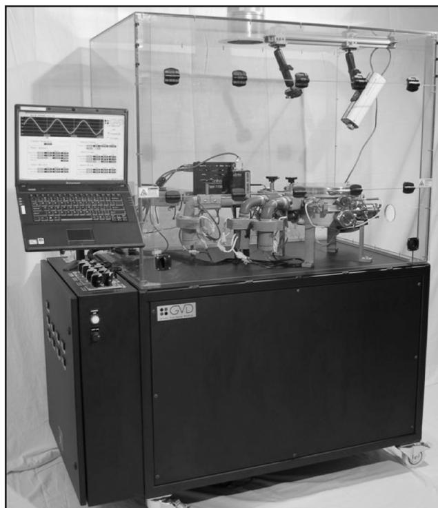
**Figure 2.** The integrated iLab chemical vapor deposition experiment at UConn. Photo courtesy of GVD Corporation.
