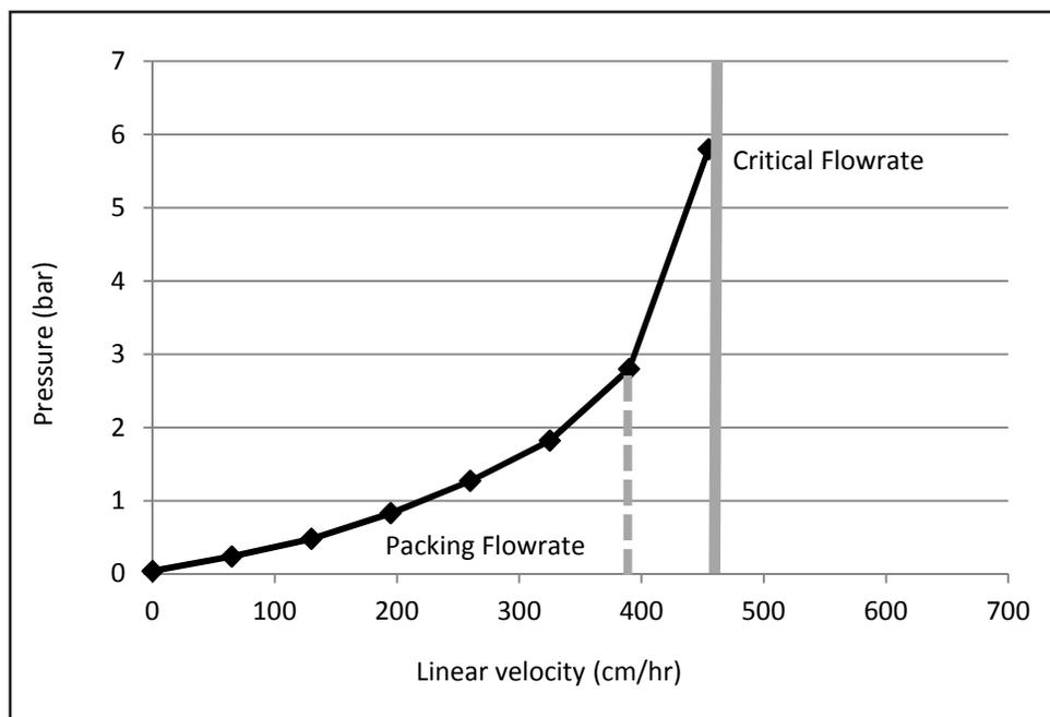
**Figure 4.** Pressure-flow curve to determine packing flow rate. The critical flow rate, defined as the flow rate at which the slope becomes infinite, was measured as approximately 450 cm/hr; higher linear velocities could not be achieved due to pressure limitations of the column. The packing flow rate is calculated as 85% of the critical flow rate.<sup>[16]</sup>
