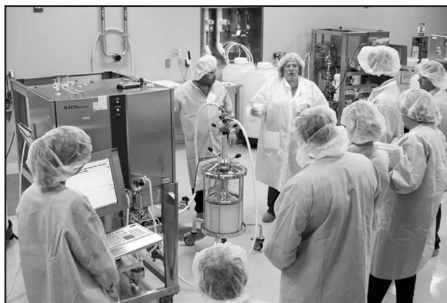
**Figure 1.** An AKTApurify™ system (GE Healthcare), located in BTEC’s large-scale process area, used in the “cGMP Downstream Operations” course.
