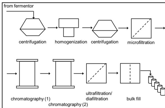
**Figure 2.** The BTEC downstream process for production of green fluorescent protein using *E. coli*.
