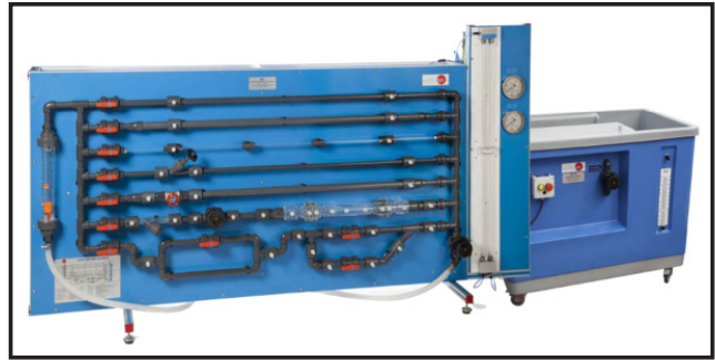
Figure 2. Edibon AFT-B Fluid Flow in Pipes equipment that is used at PVAMU Chemical Engineering Laboratory.
