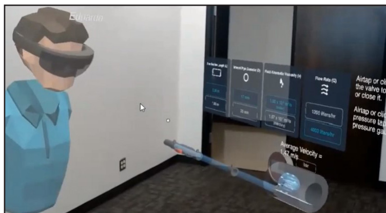
Figure 4. An example of MR used to facilitate collaborative learning between two students even though they are not physically co-located. The image is taken from the perspective of the student who is located in the lab. The avatar (left) represents the second student who is not physically present in the same space as the first student. Both students use the Microsoft HoloLens technology to view and interact with the pipe simulation digital element (right) simultaneously with no time lag.
