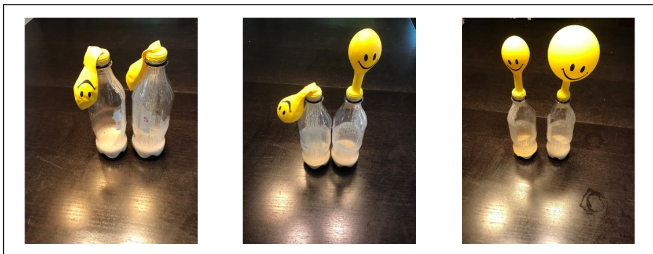
Figure 3. Photographs of experiments comparing the carbon dioxide outputs of unfed sourdough and sourdough fed with sugar. Right bottle: sourdough fed with 1 teaspoon of sugar. Left bottle: not fed. Timepoints taken at 0, 6, and 22 hours (from left to right in the figure). Students used measurements from these experiments to determine that their sourdough culture had a 1.68% yield on sucrose fed using material balances.
