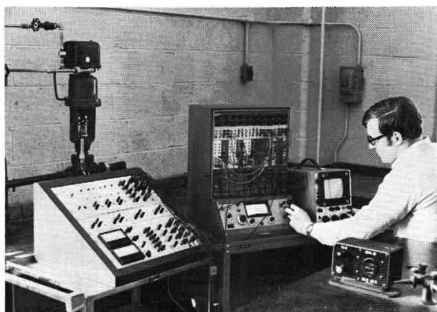
Fig. 5. Photograph Showing a System Consisting of a Pneumatic Control Valve, a Portable Interface Panel to the IBM 1800 Computer and a TR-10 Analog Computer being used in a Real-Time Simulation by an Undergraduate Student.
