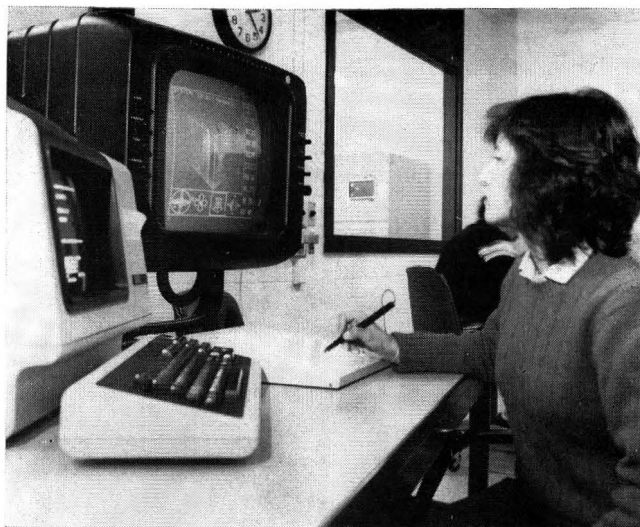
FIGURE 1. An example of a typical workstation showing the Evans and Sutherland vector refresh graphics monitor with VT100 terminal, electronic tablet and stylus.
