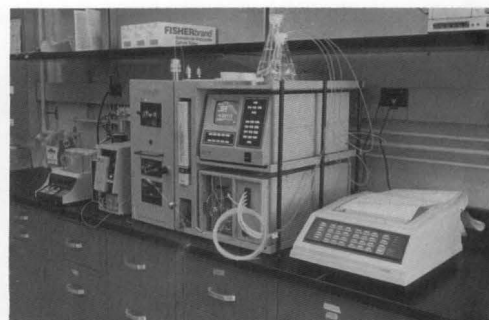
An unattended experiment? Not to worry. This machine (Cramer's new Delta Prep chromatographic unit) practically runs itself.
