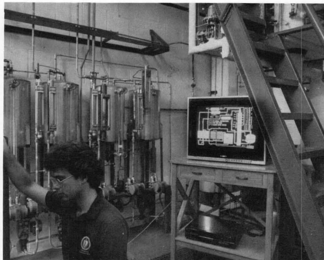
Setting up the distillation column for a steady-state experiment. Distillation column is seen on the right as is the computer monitor depicting the schematic for the column with temperatures and flow rates being shown dramatically at the appropriate positions on the diagram.
