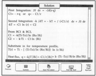
Figure 5. Solution card, initially blank, showing the completed solution for the selected problem.
