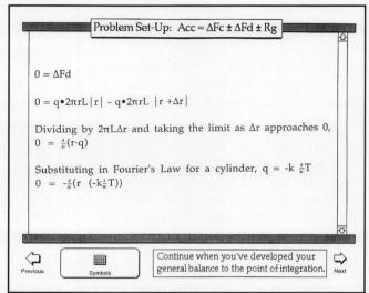
Figure 3. Problem Set Up card, initially empty, showing how to set up the problem using shell balances.
