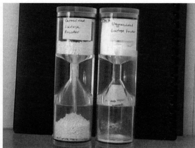
Figure 4. Granulated powder (left-hand side) flows easily into lower hopper, whereas raw powder arches and does not flow (right-hand side).
