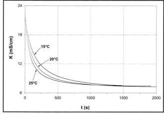
Figure 1. Conductivity of the reaction mixture in the batch reactor, as a function of time, at different temperatures.
