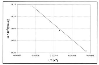
**Figure 2.** Arrhenius plot of the reaction rate constants for the second-order reaction between ethyl acetate and sodium hydroxide.
