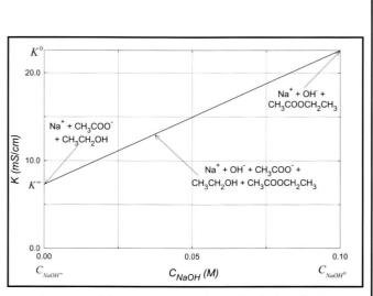
**Figure 6.** Calibration curve for the method of analysis conductivity of the reaction mixture versus the sodium hydroxide concentration.
