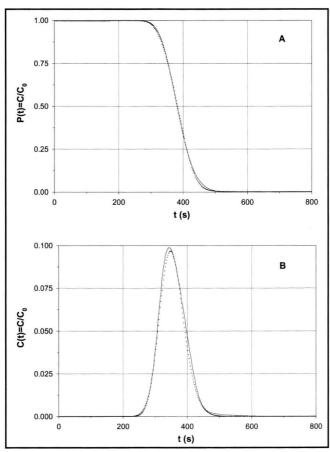
Figure 3. KCl normalized concentration data at the outlet of the packed-bed tubular reactor for (A) a negative step, and (B) a pulse input. The lines represent the fittings obtained using Eqs. (4) and (9), respectively. The fitted parameters are shown in Table 1.
