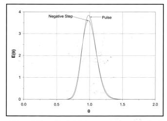
Figure 4. Normalized RTD function for the packed-bed tubular reactor based on the negative step and pulse experiments (Pe values are shown in Table 1).
