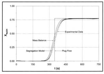
**Figure 5.** Sodium hydroxide conversion at the outlet of the tubular reactor. The lines were obtained using the total segregation model and the mass balance explained in Appendix B (with Pe = 158.7 and  $\tau = 348.3$  s).
