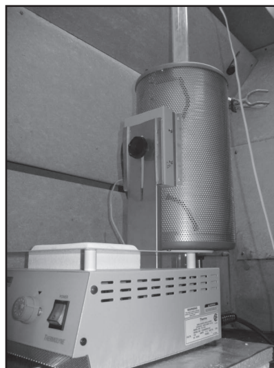
Scheme 2. Depiction of experimental setup. Quartz tube reactor within vertically mounted tube furnace.
