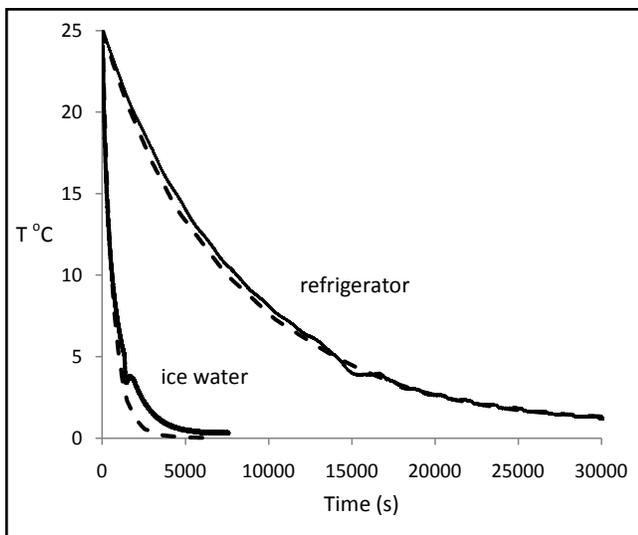
**Figure 4.** Comparison of cooling rates for glass bottle in refrigerator or ice water. Solid lines, experimental data. Dashed lines, equivalent stagnant layer conduction models.
