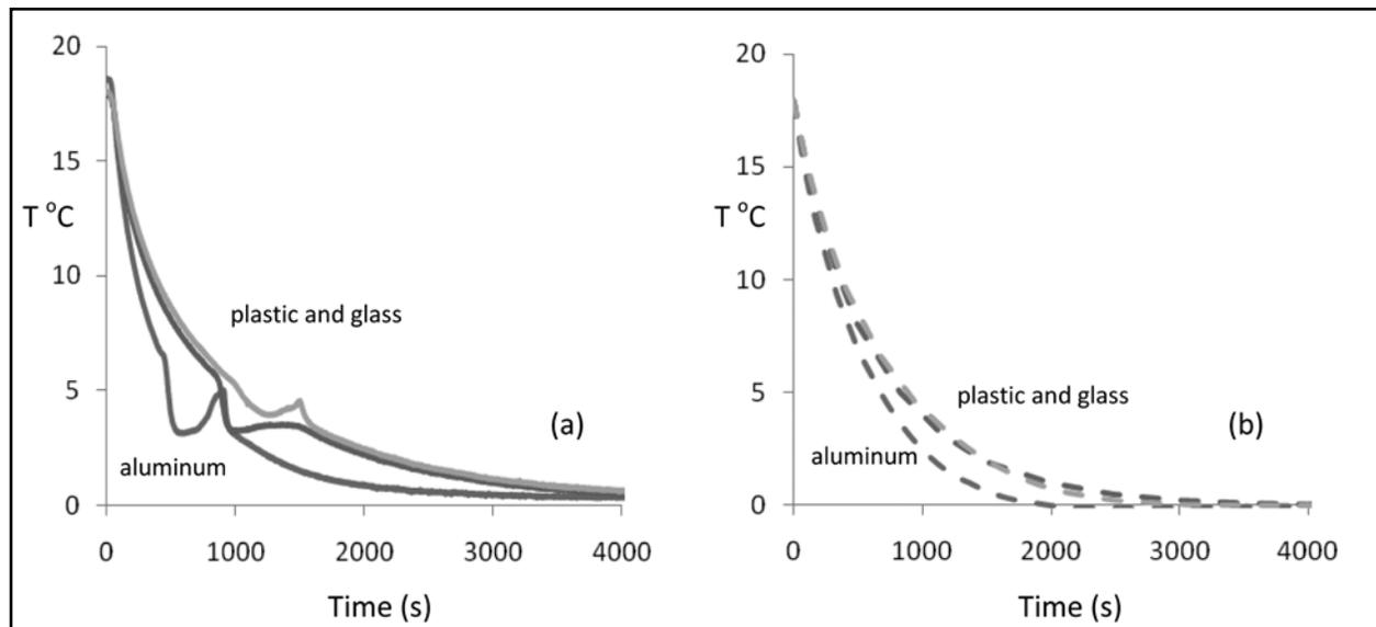
**Figure 6.** Comparison of aluminum, glass, and plastic bottles upon cooling in ice water. (a) experimental results; (b) predicted results with  $h_o = 200 \text{ W/m}^2\text{K}$ ,  $h_i = 400 \text{ W/m}^2\text{K}$ .
