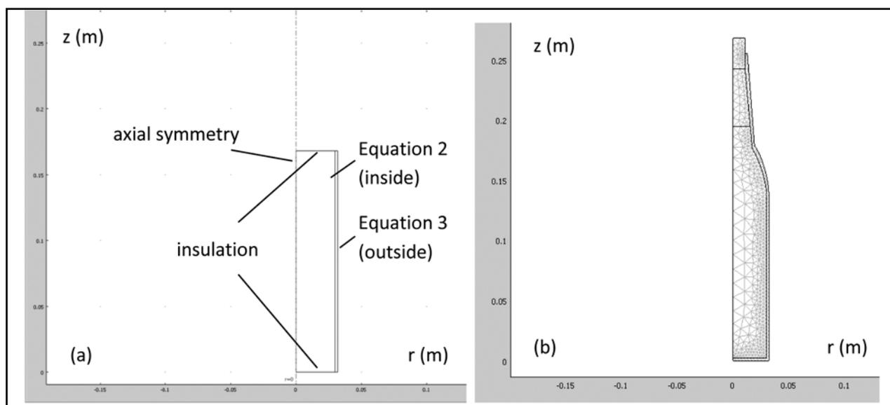
**Figure 1.** 2-D axially symmetric geometry of glass bottle modeled as (a) equivalent cylinder filled with water, and (b) more realistic bottle shape with air between water and rubber stopper. Boundary conditions are indicated on the equivalent cylinder model.
