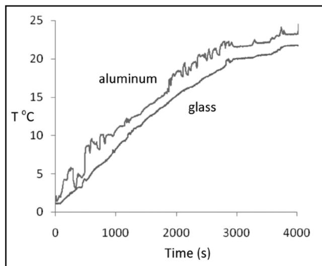
**Figure 7.** Hand-held heating experimental results for glass and aluminum bottles.
