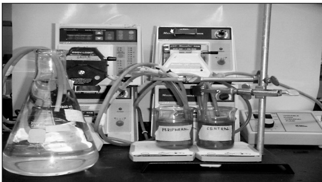
Figure 2. The experimental setup of the two-compartment model. Potassium permanganate was added to the beakers. Fresh water in an Erlenmeyer flask was introduced to the two compartments.
