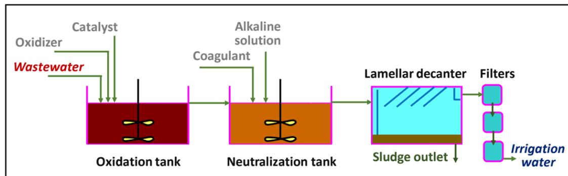
Figure 2. Fenton-like oxidation flow-scheme.
