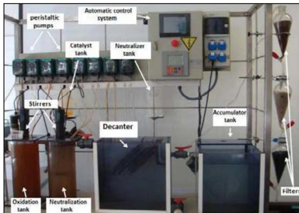
Figure 3. Fenton-like oxidation pilot-scale plant.
