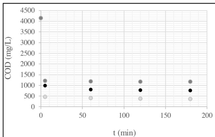
**Figure 4.** COD concentration in the Fenton oxidation CSTR vs. time. Experimental conditions  $[Fe^{3+}]/[H_2O_2]$  ratio: = 0.02 (dark gray dot), 0.09 (black dot) and 0.2 (light gray dot); pH = 3 and temperature 20 °C.
