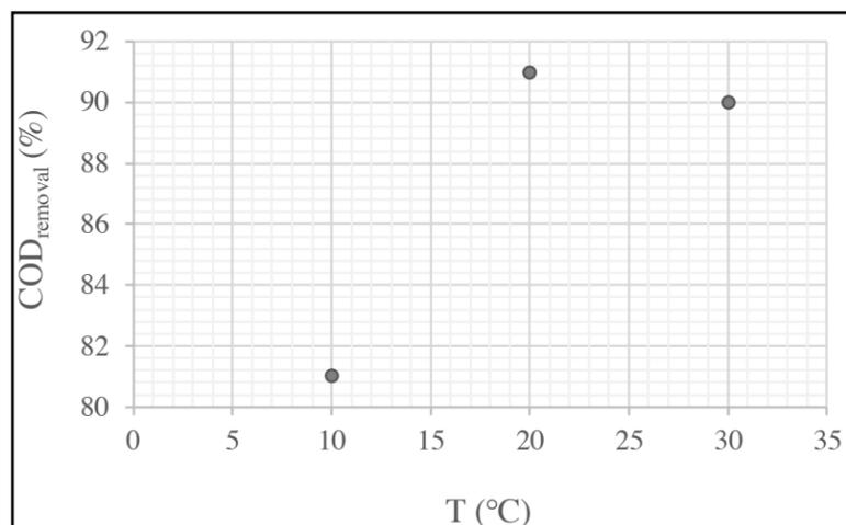
**Figure 5.** COD removal efficiency in the Fenton oxidation CSTR vs. T: 10, 20, and 30 °C. Experimental conditions:  $[H_2O_2] = 45$  g/L,  $[Fe^{3+}] = 4$  g/L, pH = 3.
