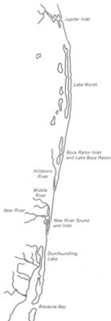
Natural waterways along the southeast Florida coast as they appeared in 1889. This series of inlets, rivers, and lakes was connected to form the Florida East Coast Canal, today's Intracoastal Waterway.
