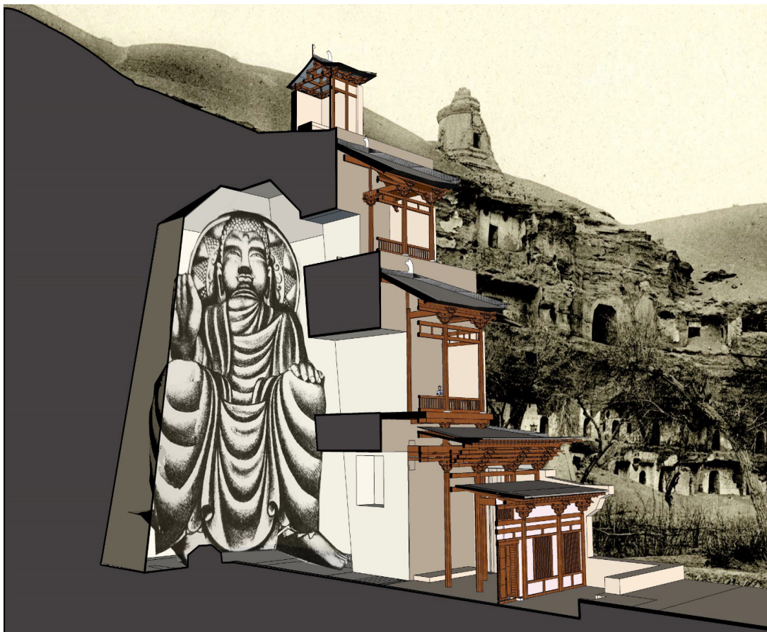
Figure 12. Theoretical reconstruction of the composite cave-front architecture of Mogao Cave 130, cave constructed in early 8th century, and pavilion in 10th–11th century. Design and drawing by author.
