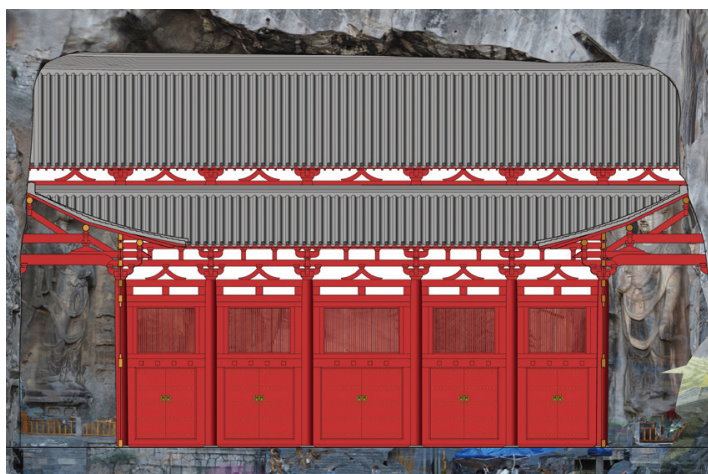
Figure 9. Traces of beam holes in-between the colossal images (left) and a theoretical reconstruction of the timber structure screening the Fengxian Temple of the Longmen Grottoes, showing a double-eave timber porch with two corridors on the sides. Design and drawing by Li Ruoshui. After Peng and Li, "Longmen fengxian si da lushena xiangkan tangdai de buzao yu jiajian," 114–115, figs. 5, 7.
