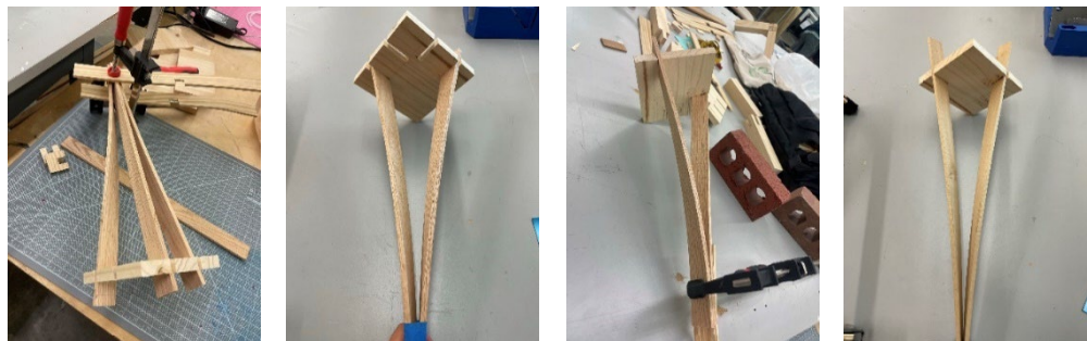
Figure 11. Steam Bending Corner Mock-Ups
