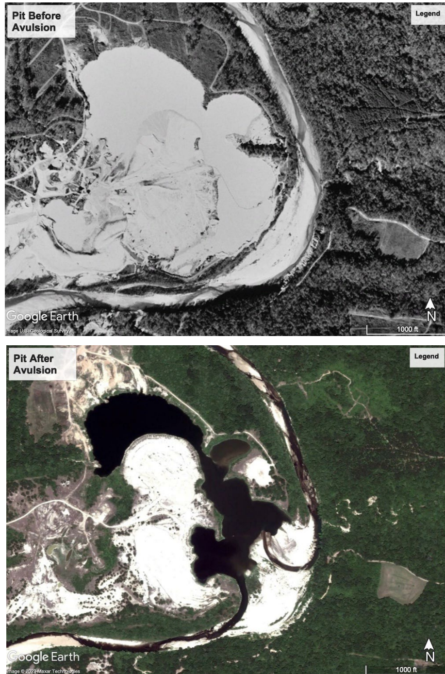
Figure 2. Section of Bayou Sara, Louisiana, before and after pit avulsion.
