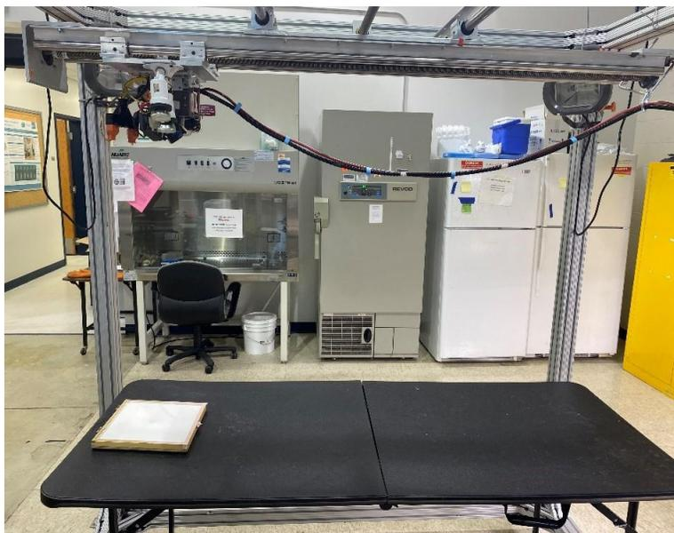
**Figure 1.** SPOT Facility Including Reflectance Panel, Camera, Lights, and Table
