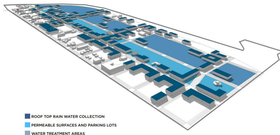
Figure 5: Proposed redevelopment water infrastructure design in Bend, Oregon. Reprinted from A Living City/Bend, Oregon , by R. Graves and J. Fisher, 2014, p. 93. Copyright 2014 by The International Living Future Institute.
