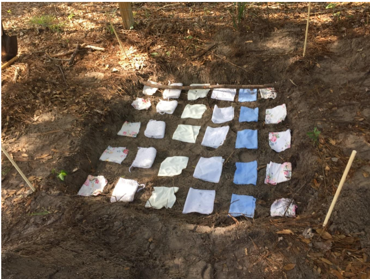
Figure 2: The layout of each site, using Site 1 as an example. From left to right the textiles present are: UV-protected cotton, wool, polyester, ripstop, cotton-polyester blended fabric, and cotton.
