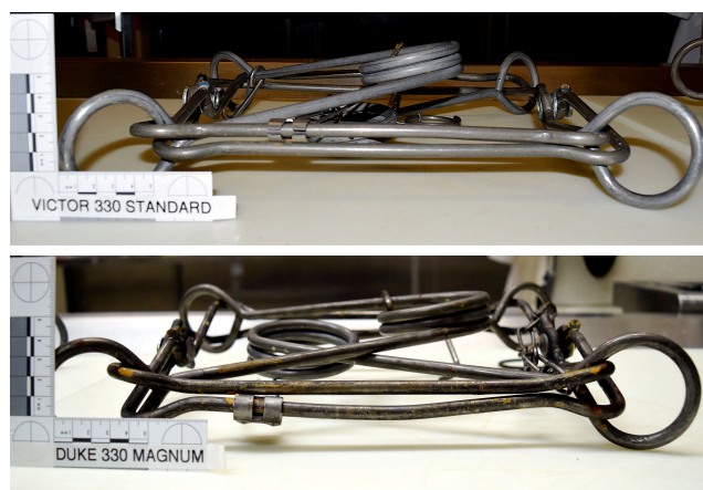
FIGURE 2—Jaw gaps. The gap in the closed jaws, measured at the midpoint, of the standard bodygrip 330 trap (top) was 4.5 mm; the Magnum bodygrip 330 trap (bottom), 6.0 mm.
