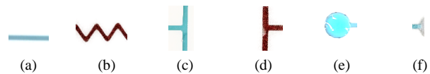
Figure 1 Real images of fundamental elements filled by die water or blood, a) Straight Channel, b) Zigzag Channel, c) Splitting Joint, d) Merging Joint, e) Inlet, f) Ventilation.
