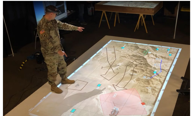
Figure 2: Combination of display technologies utilized simultaneously, including live sand (back), ground projection (center), and head mounted display (worn)
