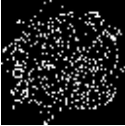
Figure 3: I/Q Image from 64-QAM
