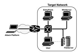
Figure 4: The evaluation network. The dotted line represents a Firewall rule that restricts access to the **FileServer** host from the **User** host.
