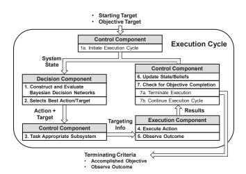
Figure 1: The Control Logic flow of execution.
