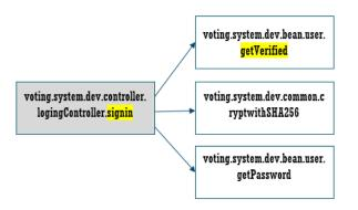
The extracted path from the source code of the authentication process is: { signin, getVerified, signin-completion }
