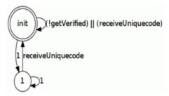
"!getVerified " means any event but getVerified, and ( $\mid$  ) is utilized to match either not getVerified or receiveUnique-Code.
