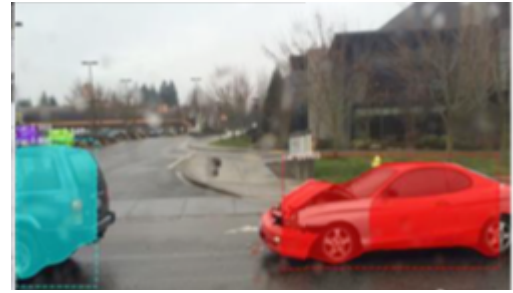
Figure 5 Vehicle detection result of another sample image
