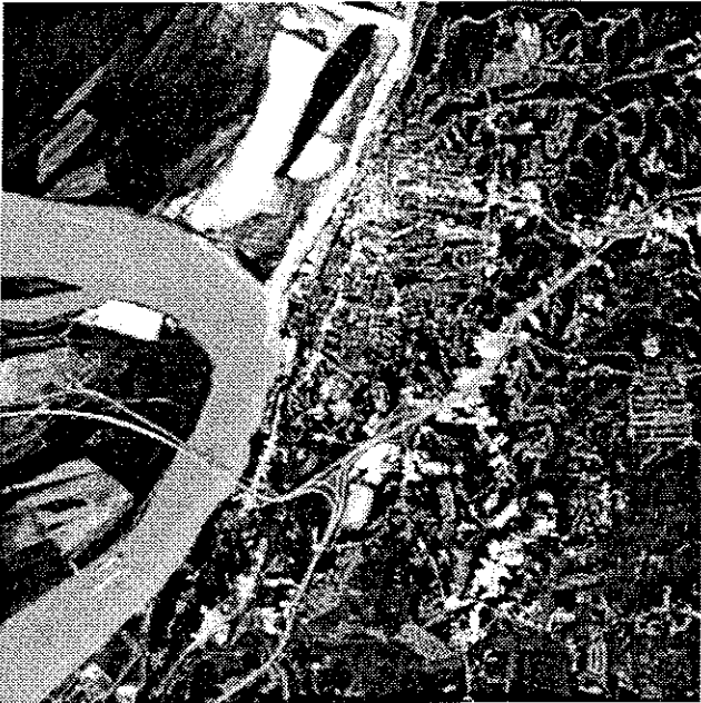
LandSat Thematic Mapper Satellite Image of Vicksburg, Mississippi: Channel 3, Histogram Equalized Figure 1
